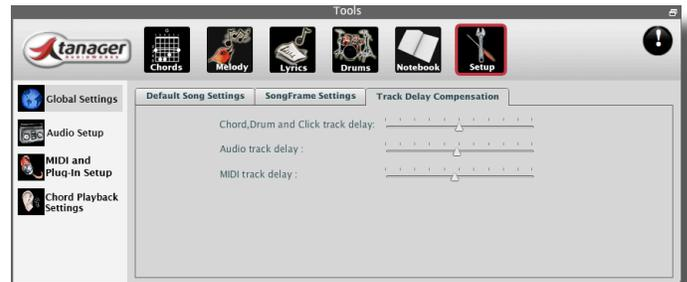
As you begin recording audio in the Audio Track, playback may be slightly delayed. Slide the **Audio Track Delay** slider to the left a bit as shown to play the audio back sooner in relation to the MIDI tracks. Adjust this until your system timing is aligned properly. The **MIDI Track** slider can be used to optimize the playback sync of the Melody/MIDI track.
